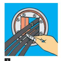
Pull the cables to final position. Mark cable 30 mm from front edge of frame. Remove cable sheat 5 mm on either side of the line.
