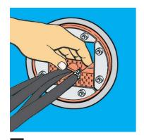
When packing the transit, ensure all the insert blocks have "E" markings thread is visible.
