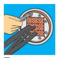
Tighten the nuts so that 10-12 mm of the protruding thread is visible.
