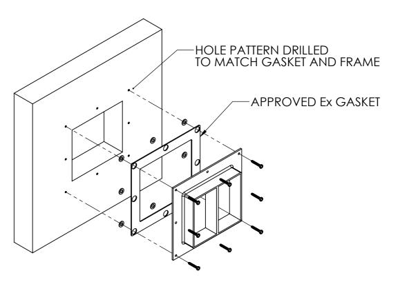
This typical installation drawing is valid for all frame types and combinations.
