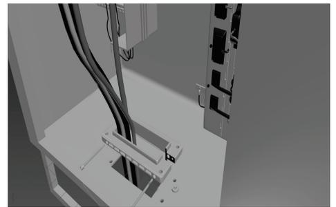
**15. Install the preterminated cables between the two halves of RFCS frame.**
