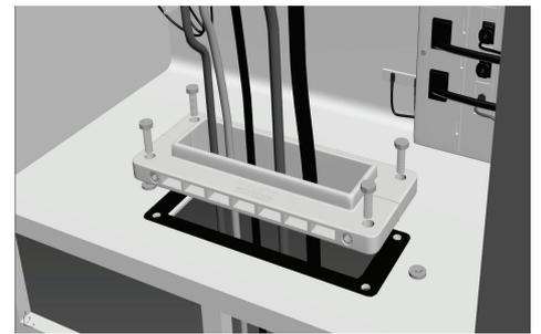
**18. Fix the RFCS frame together with back gasket on the cabinet cutout by tightening with mounting hardware.**
