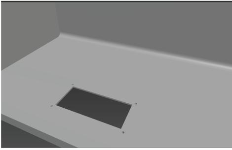
1. Start the installation by ensuring that the cutout made in cabinet correspond to the cutout pattern in the installation manual.
