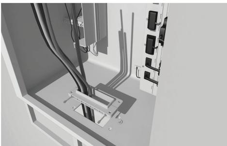
**16. Screw together the two halves with middle gasket fixed on one half of the RFCS frame.**
