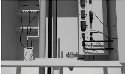
**11-12. Tighten the PTG 40 wedge until it is almost even with the frame surface to obtain IP 65/67 rating.**
