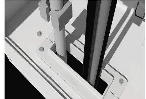
6. Install the cable within the prepared halves of CS module.
