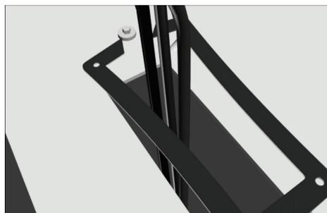
**17. Install all preterminated cables after making an angular cut in the gasket and secure the gasket on cabinet cut out.**
