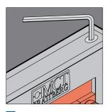
Insert compression system and tighten using allen key.
