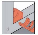
**5** Detach sealing rings from main block and retain ring corresponding to measured cable size. In this example 26 mm.
