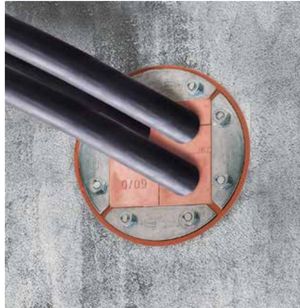
RGP transit placed in a drilled hole. No compression plate or final seal is required
