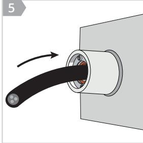
Install the sealing into the SR housing and guide the cable or pipe through it.
