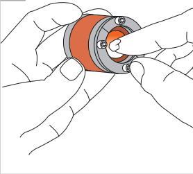
Lubricate the inner sealing surfaces and the cable or pipe using MCT Brattberg Lubricant.
