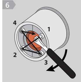
Gradually tighten the screws in a crosswise pattern until the cable or pipe is securely fixed and the rubber seal protrudes slightly.
