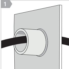
If the cable or pipe is already installed, open the SR sealing and place it over the service.
