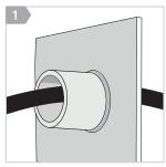
If the cable or pipe is already installed, open the SR sealing and place it over the cable or pipe.
