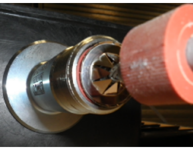
Slide 2nd piece of Seal Over cable
