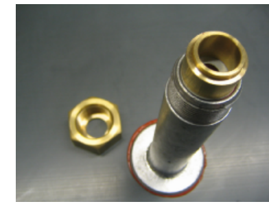
Fit Washer if required and next add Compression Spigot
