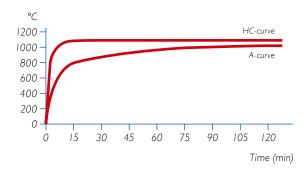
For example, a penetration that withstands an H-Class fire for 120 minutes is classed as H120 and a penetration that withstands an A-Class fire for 60 minutes is classed A60.
